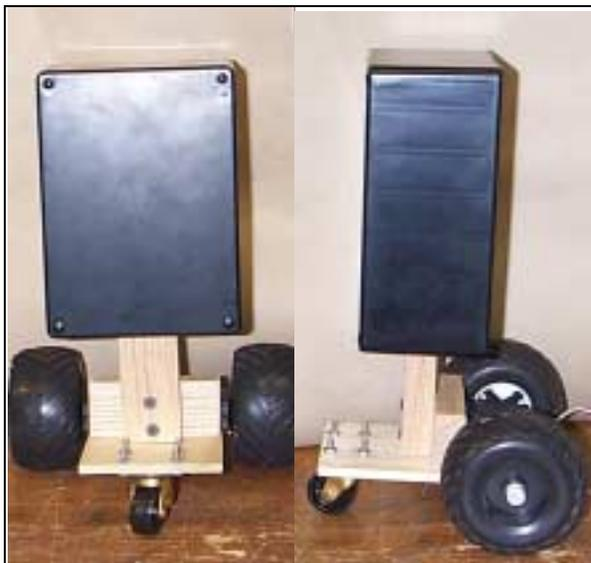
These pictures show my fighting robot body design with the project box mounted away from the drive servos. You can of course simple mount servos right onto the project box. To mount servos or other drive motors inside a project box you'll need to drill a starter hole in the box. You'll then need a good strong utility knife to cut away the rest of the plastic to make the correct cut out size for your servo or other drive motor device.
