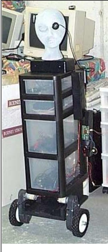
Here is a new idea for a robot body, use a draw cart. The robot pictured to the left is named Borg 1-of-1. It's going to be my computer controlled robotics platform for testing. The main goal of this robot is to play around with some security robot ideas that I have. The robot has a servo-controlled arm, which can raise and lower a hacked "laser tag" toy. This will allow me to play laser tag with my robot.
