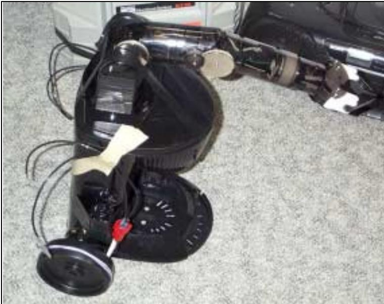
After removing all of the electronics and heating elements. What I was left with was a great looking robotics shell. Where the electronic controls were is now perfect for mounting an LCD or different sensor arrays. The flitter area provides a great little electronics bay, which is hinged and can swing out. Where water used to go in could now hold batteries or motor controls, just about anything.
