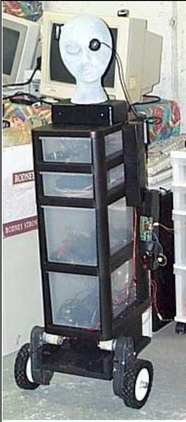
Here is a new idea for a robot body, use a draw cart. The robot pictured to the left is named Borg 1-of-1. It's going to be my computer controlled robotics platform for testing. The main goal of this robot is to play around with some security robot ideas that I have. The robot has a servo-controlled arm, which can raise and lower a hacked "laser tag" toy. This will allow me to play laser tag with my robot.
