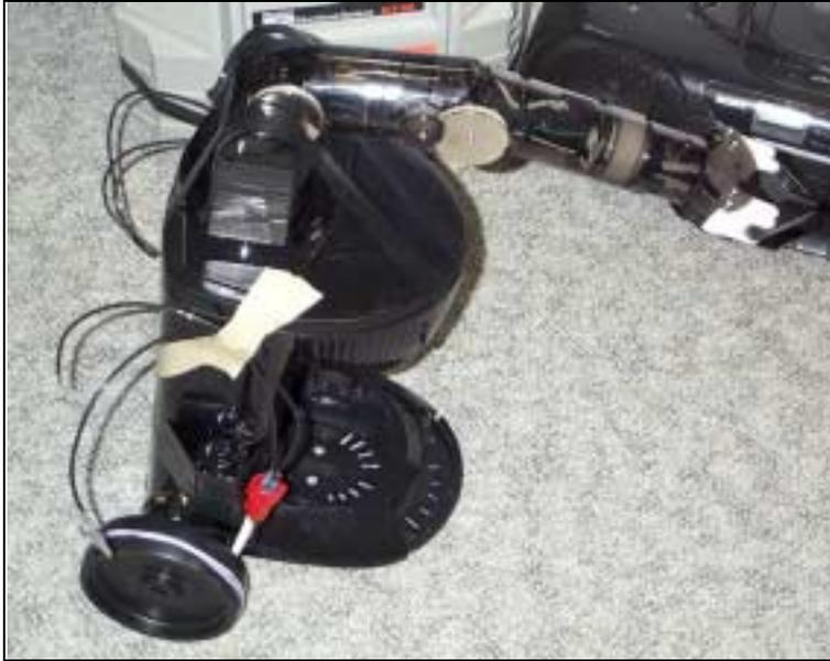
After removing all of the electronics and heating elements. What I was left with was a great looking robotics shell. Where the electronic controls where is now perfect for mounting an LCD or different sensor arrays. The flitter area provides a great little electronics bay, which is hinged and can swing out. Where water used to go in could now hold batteries or motor controls, just about anything.
