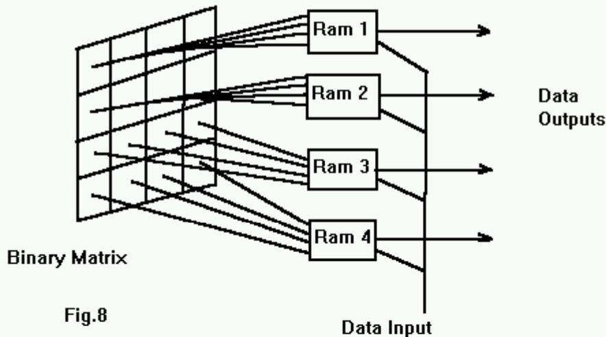
Each memory element has an N-Bit address field. In this case N=4 Each memory element samples its N-Tuple of sub pattern in the binary matrix, and this is the address for each memory element. I will use SRAM's for my experimental robot. Each layer of memory elements covers the binary matrix once and is known as a discriminator.
