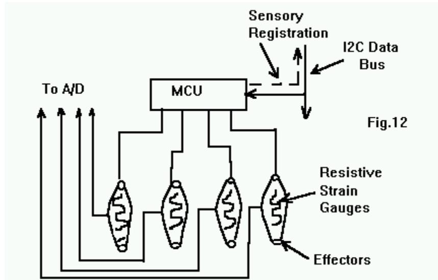
All of the mcu's are connected together by an I2C data bus. This bus carries control signals from the mcu's to the effectors. It also carries interoceptors information from the mcu's to the heuristic processor. Control signals take the following form:
