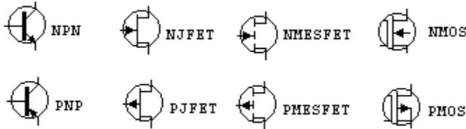
The two schematic symbols for basic bipolar transistors are shown to the far left with the labels NPN and PNP. A small current going to the emitter and base of these transistors will cause a much larger emitter and collector current to flow.
