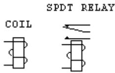
Relays are electromagnetic switch. Small current flows through a coil in the relay, which creates a magnetic field that pulls the one switch contact towards or away from another. Relays are pretty common; in fact when you signed online you probably heard the click of a relay right before your modem dialed up you internet connections!
