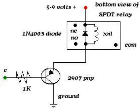
The emitter is the transistor pin that is connected to the ground. The Base is the pin going to the 1K resistor and the other pin is the collector. A data pin from your computer's printer port could connect to other end of the 1K resistor (marked C). You would also need a ground from the computer printer port to complete this circuit. I want to point out the relay in the picture was drawn by hand fully illustrate the pin out from the bottom of the relay.
