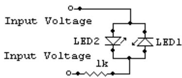
An LED can stop current flow like any normal diode. The schematic to the left shows a voltage indicator. You can apply a positive and negative voltage to the points labeled "input voltage." If you switch the order of positive and negative the opposite LED will light.
