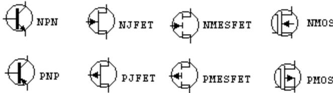
The two schematic symbols for basic bipolar transistors are shown to the far left with the labels NPN and PNP. A small current going to the emitter and base of these transistors will cause a much larger emitter and collector current to flow.
