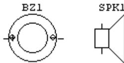
BZ1 is the common schematic symbol for a buzzer. SPK1 stands for speaker1 and is the common symbol for a speaker. The "1" is added so signify the first speaker. You'll often see a number even if there is only one component of the type used.
